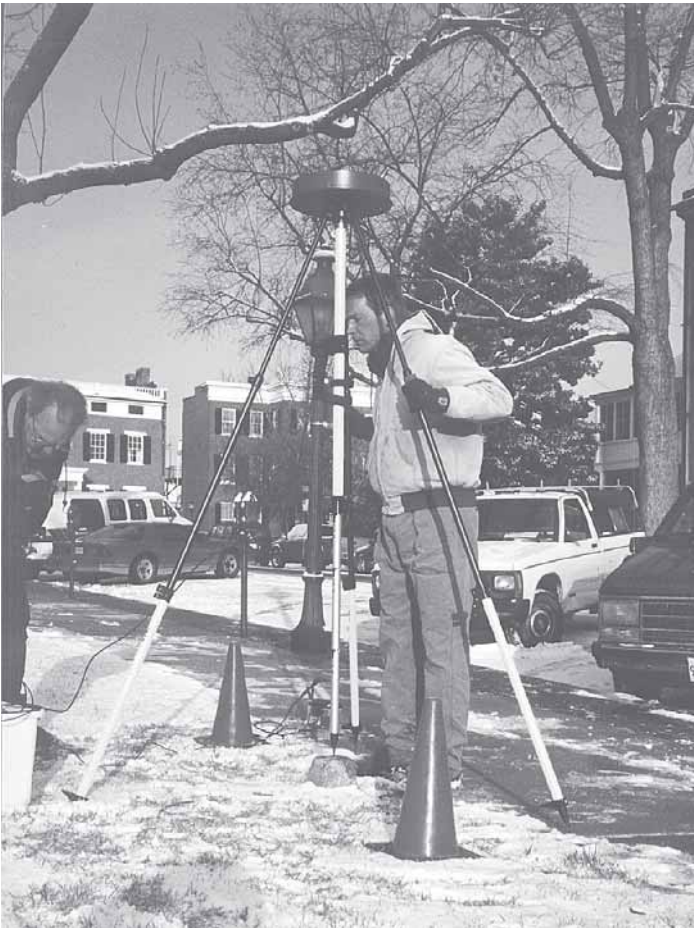
Where surveyors of old once checked their compasses, Bill Orsinger of VIKA sets up a Seco 2-meter pole with NGS choke-ring antenna, over "North Magnetic" in Frederick.
