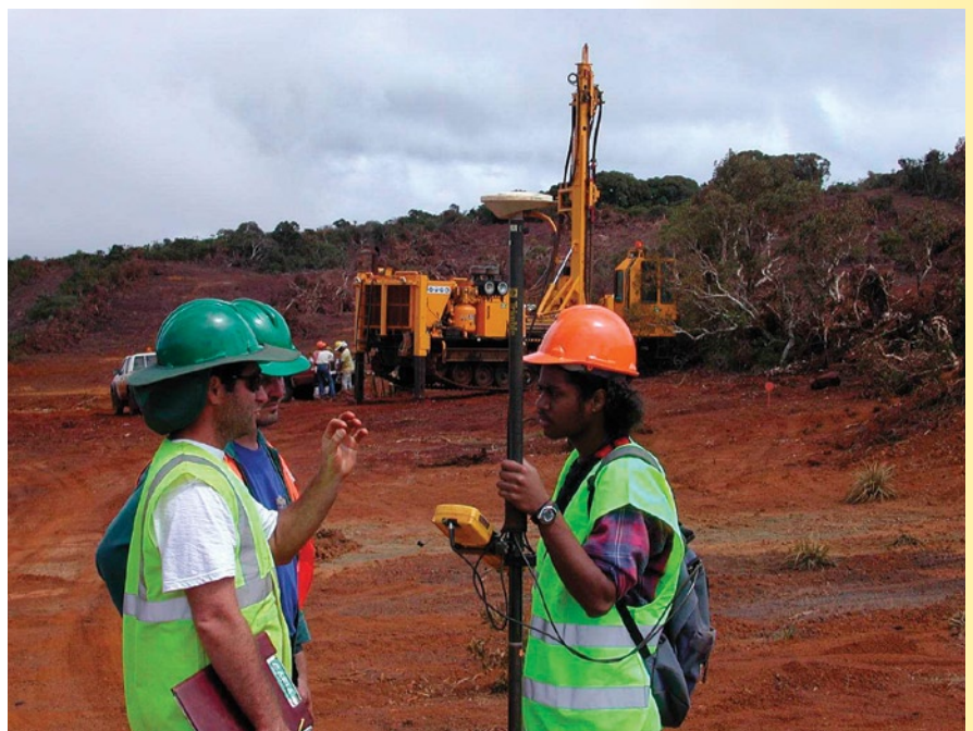
Top: The Tiebaghi Mine uses a Trimble 5700 RTK GPS system to stake out new mining limits; the system is also used daily to check the excavator's horizontal level for drainage and quality of product.
