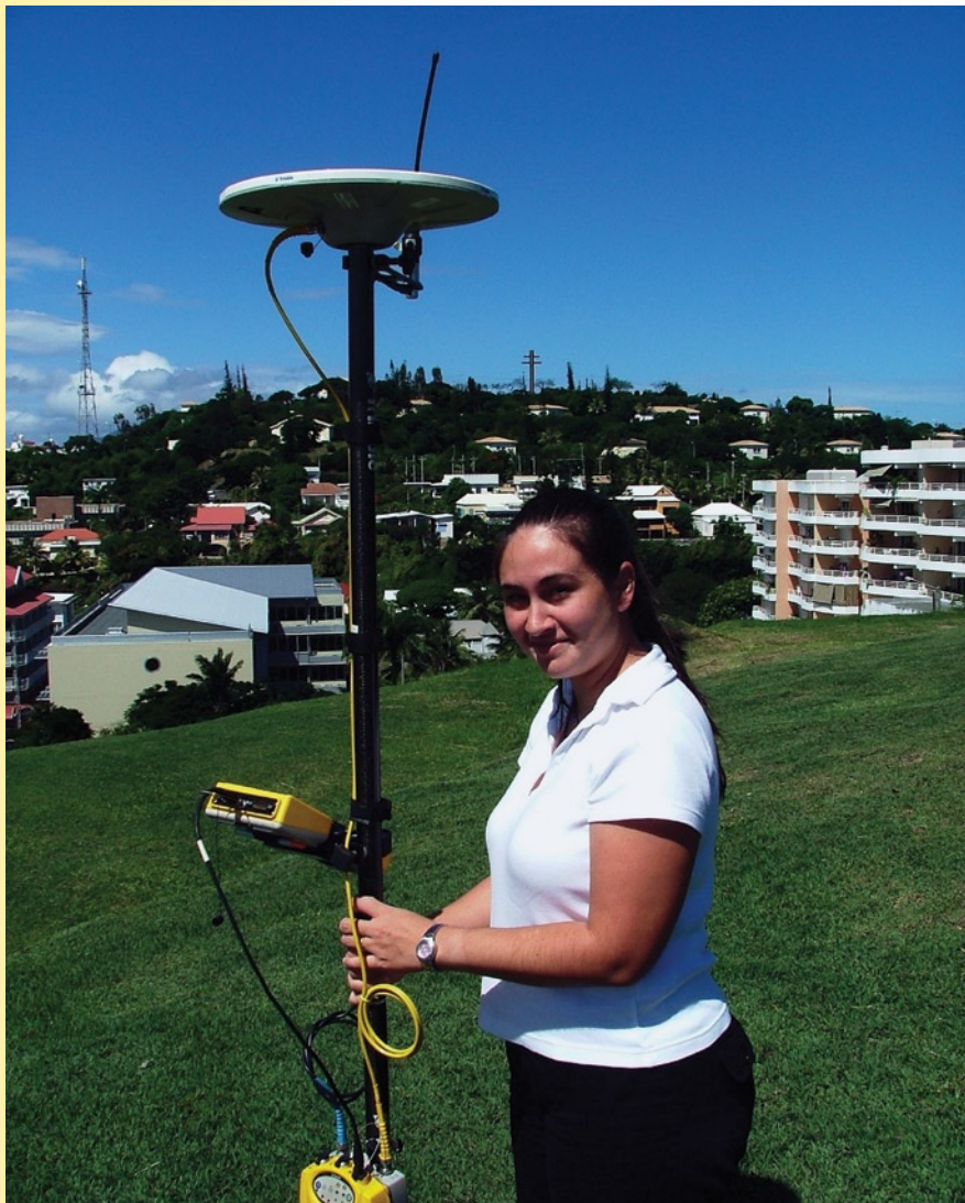
A surveyor uses a Trimble RTK GPS 5700 with TrimMark3 UHF radio system broadcast from Nouville's reference station to collect the Topo for the expansion of a residential complex at Baie de la Moselle (Nouméa).
