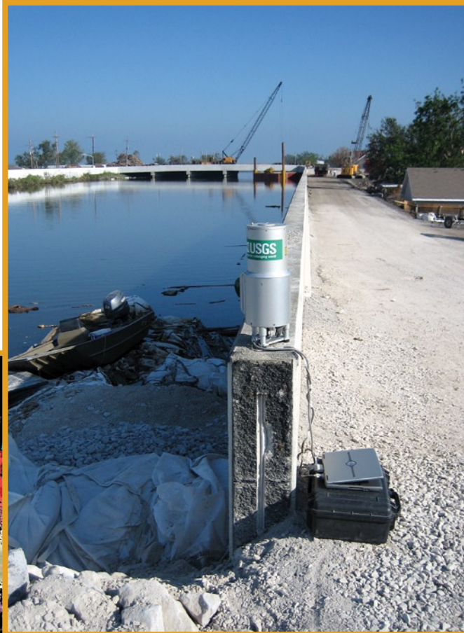
Above: LIDAR unit on the edge of intact I-wall levee at the north end of the 17th Street breach.
